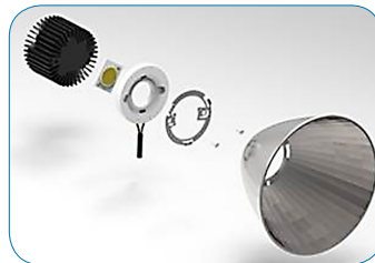
TE Type Z50 LED holder with TE optics retaining clip shown with Sharp Mega ZENIGATA LED, LEDIL optics and generic heat sink.
