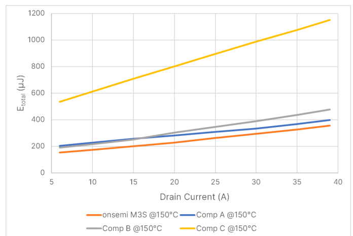
Fig.17: Total switching losses comparison at V_{DC} =400V, V_{GS} =18/-3V, R_G =4.7 \Omega
