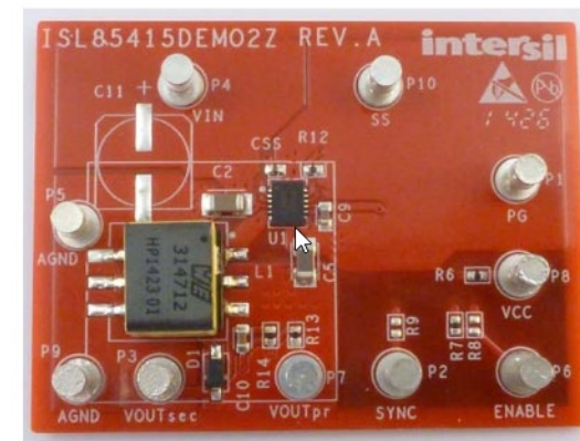
FIGURE 1. FRONT OF EVALUATION BOARD ISL85415DEMO02Z
