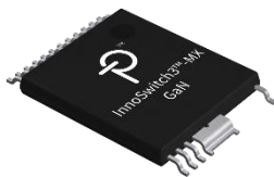
InSOP-24D (C-Package) MSL-3 rated – wave solder and reflow
