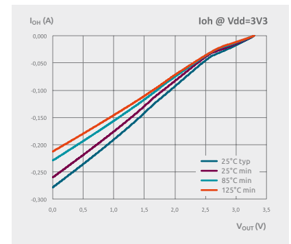
LVT output curves at 3V3
