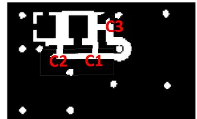
The antenna needs a matching circuit to adjust the resonant frequency balance. When delivered, the evaluation board is tuned for optimum balance at 1.575 GHz and 1.602 GHz using the following component values:
