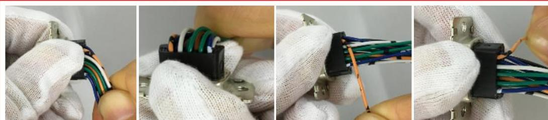
Wrong method: over-tighten & use excessive force to bend the terminal.
