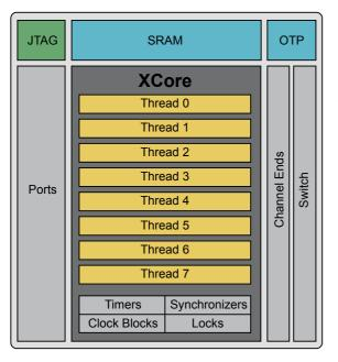
input-output and timing; this makes the cost of these operations the same as arithmetic, memory operations and branches. Each XS1 core has a single unified memory system, which is shared for program and data by all of the threads executed by the core. This means that multiple threads can share the same program in memory. Memory access is single cycle, giving high performance without caches.
