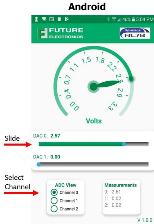
Tip: If you are trying to set 10V on DAC1 but measurements keeps are coming up short, this could mean your batteries are getting weak. If so, please replace batteries.
