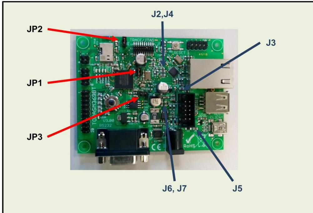
The jumpers JP1 and JP2 are normally closed. They can be opened to separate the microcontroller or the Bluetooth® module from VCC and to insert an ammeter there in order to measure current draw.
