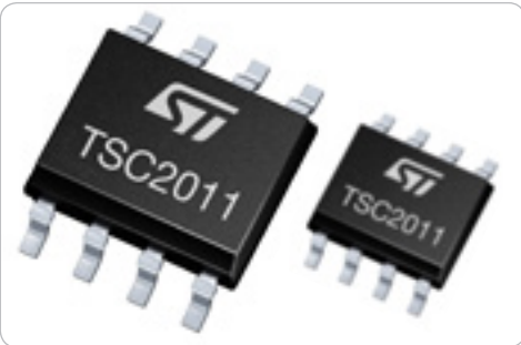
TSC2011: Performs low- or high-side current sensing
