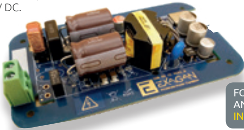
Fig. 3: The Exagan G-MODULE™ board, a 60W USB PD power adapter
