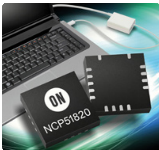
NCP51820: Low-inductance 4mm x 4mm package
