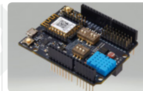
WizFi360-EVB: Compatible with the Arduino board standard
