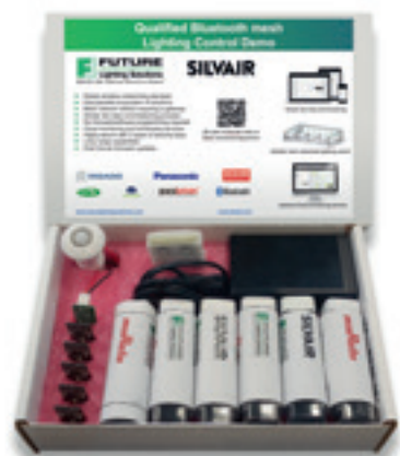
Fig. 3: The Bluetooth mesh Demo Kit from Future Lighting Solutions gives OEMs a model for the implementation of wireless control technology. (Image credit: Future Electronics)
