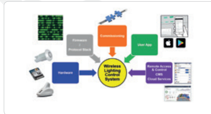
Fig. 1: The components of a Bluetooth mesh wireless lighting control system
