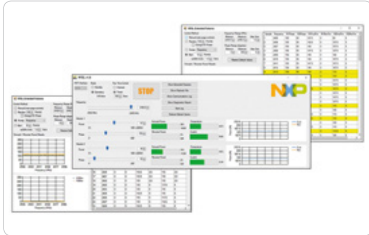
Fig. 2: NXP's Lab box RFEL software enables the user to sweep across phase and frequency to find the points with the best match to the load
