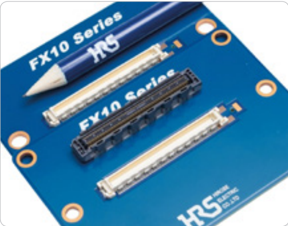
FX10 connectors: 0.5mm pitch and ±0.3mm misalignment range
