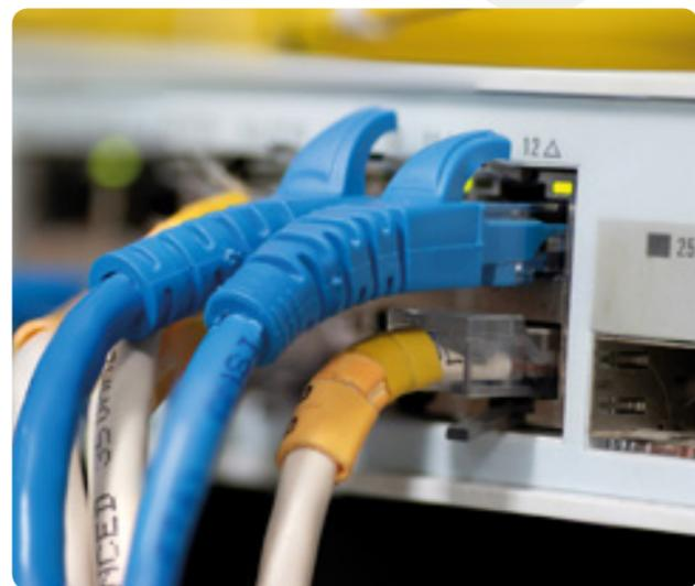
The use of a three-wire choke improves EMI performance and allows for remote powering of peripherals over the Ethernet cable. The new jacks comply with the IEEE 802.3at PoE+ standard, under which up to 25.5W of power may be supplied per port.
