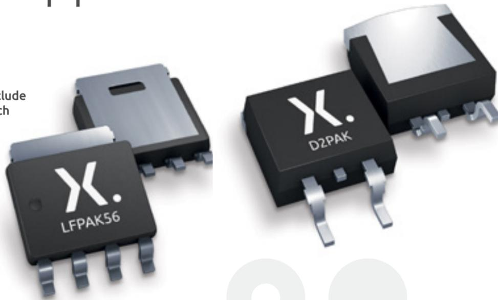
To address this problem, Nexperia has developed MOSFETs that provide an improved current-sharing capability. When used in parallel configuration, these devices remove the need for matched threshold voltage values.
