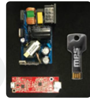
Fig. 2: The MPX2001 evaluation kit, a small design intended as a demonstration of a power adaptor or charger for a computer or smartphone.
