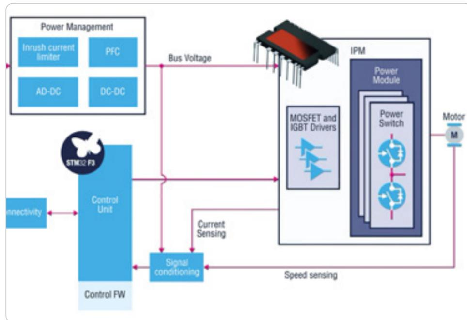
Fig. 1: Block diagram of induction motor system based on ST power and control boards
