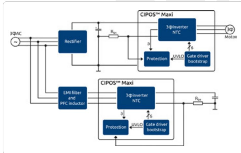
CIPOS Maxi: Typical application circuit for a three-phase motor's power stage
