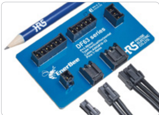
DF63: Multiple connectors may be mounted side-by-side
