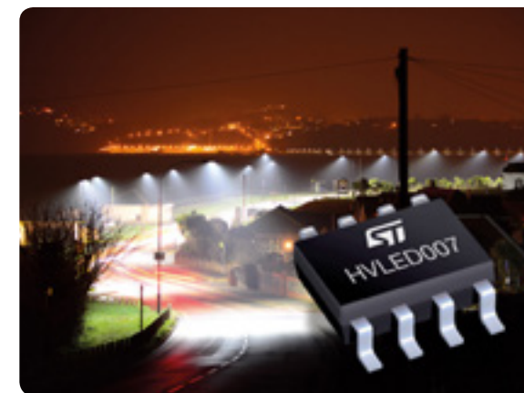
HVLED007: For use with isolated flyback converters
