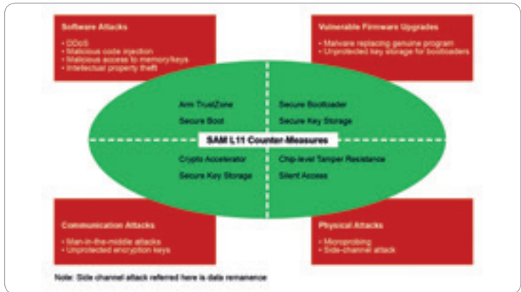
Fig. 3: The SAM L11 MCU's comprehensive security features protect against various forms of attack. (Image credit: Microchip)
