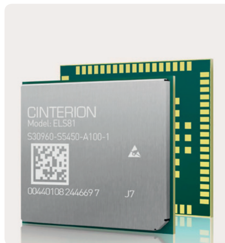
ELS81: Built-in TCP/IP stack
