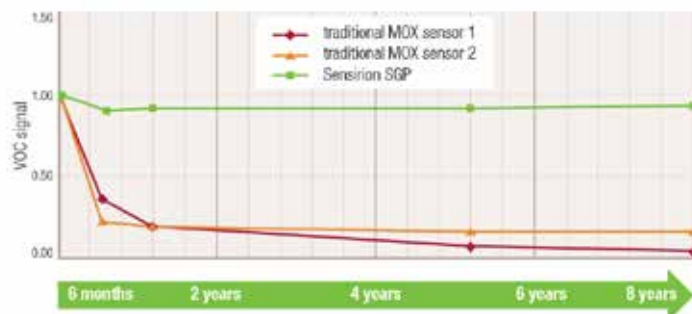
Figure 2: Testing long-term stability of MOX Sensors (Source: Sensirion)
