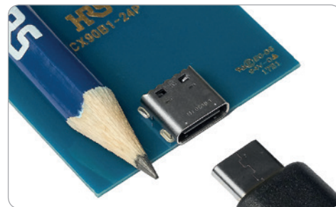
CX series receptacle: Symmetrical mating face
