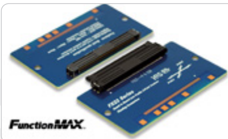
FX22: Self-cleaning function on contacts
