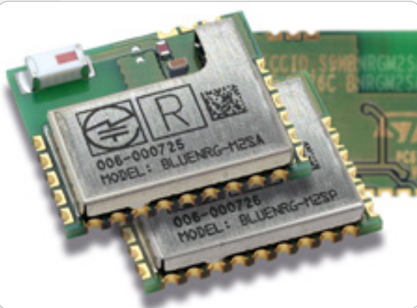
BlueNRG-M2 module: Integrated antenna and supporting circuitry
