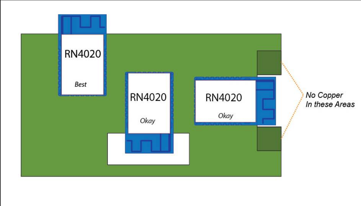
FIGURE 4-4: RN4020 HOST PCB EXAMPLE LAYOUT
