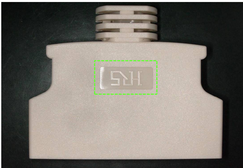
HQS mark appearance by replaced mold
