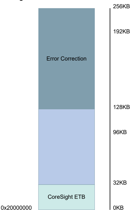
Figure 9-3. Memory with ECC and CoreSight ETB
