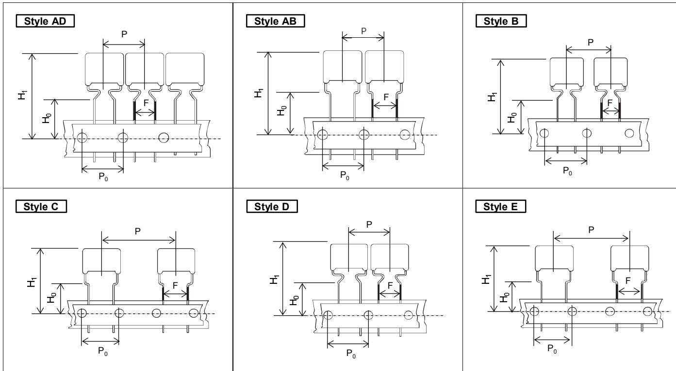
\*: H1 dimension is based on insertion machine "Panaser RH series" made by Panasonic.
