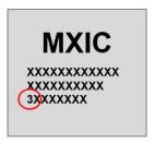
3)Package Label outside of shipping box can also identify the wafer Fabs. Lot# can be identified on the label. Lot# starts with number "2, 3, or 5" means the device is from Fab 2, whereas Lot# starts with number "7,8, or 9" means the device is from Fab 5 (Please refer to the below label illustration as an example, lot# starts with a "3" means it is from Fab 2)
