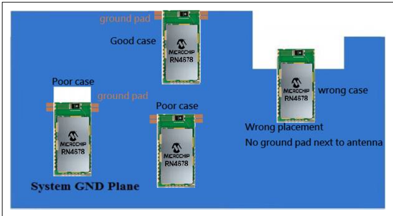
FIGURE 7-1: MODULE PLACEMENT EXAMPLES
