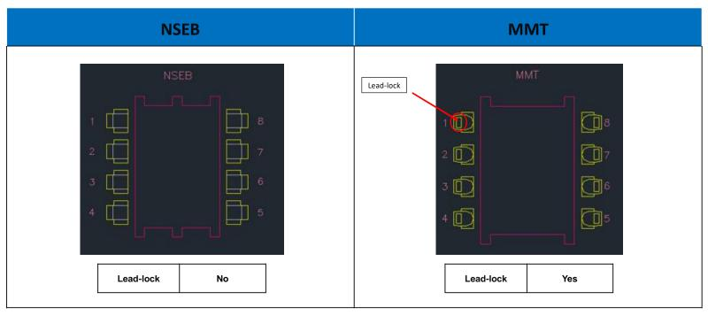
Note: Mold compound material fills the lead-lock hole, which provides improved protection against moisture penetration along the edge of the leads (pins) of the package.
