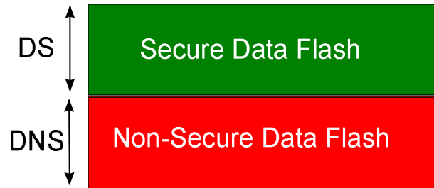
Figure 12-3. PIC32CM LS00/LS60 Data Flash Memory Mapping
