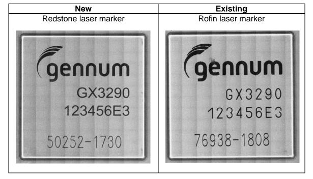
The marking quality of both pieces of equipment is comparable. The new marking has been inspected and tested, and it complies with all of Semtech's marking requirements and specifications.
