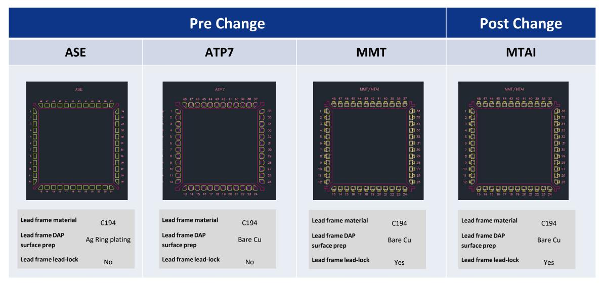
Note: The lead lock hole fills with mold compound during the assembly process and provides improved protection against moisture penetration around the interface edges between pins and mold compound.
