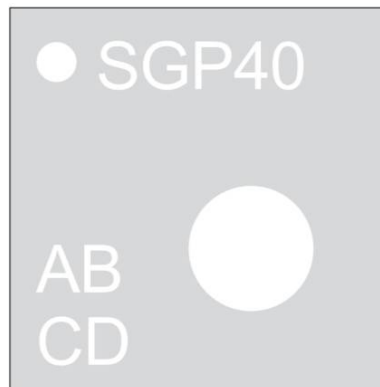
Figure 12 Top view of the SGP40 illustrating the laser marking.
