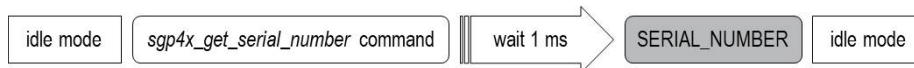
Figure 10 Process flow for reading out the serial number of the SGP40 sensor.
