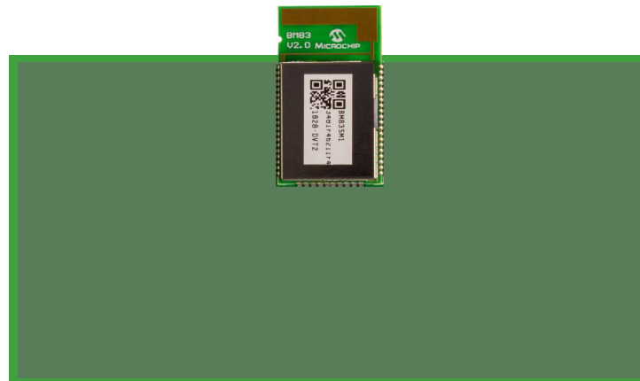
Figure 7-5. Recommended Module Placement
