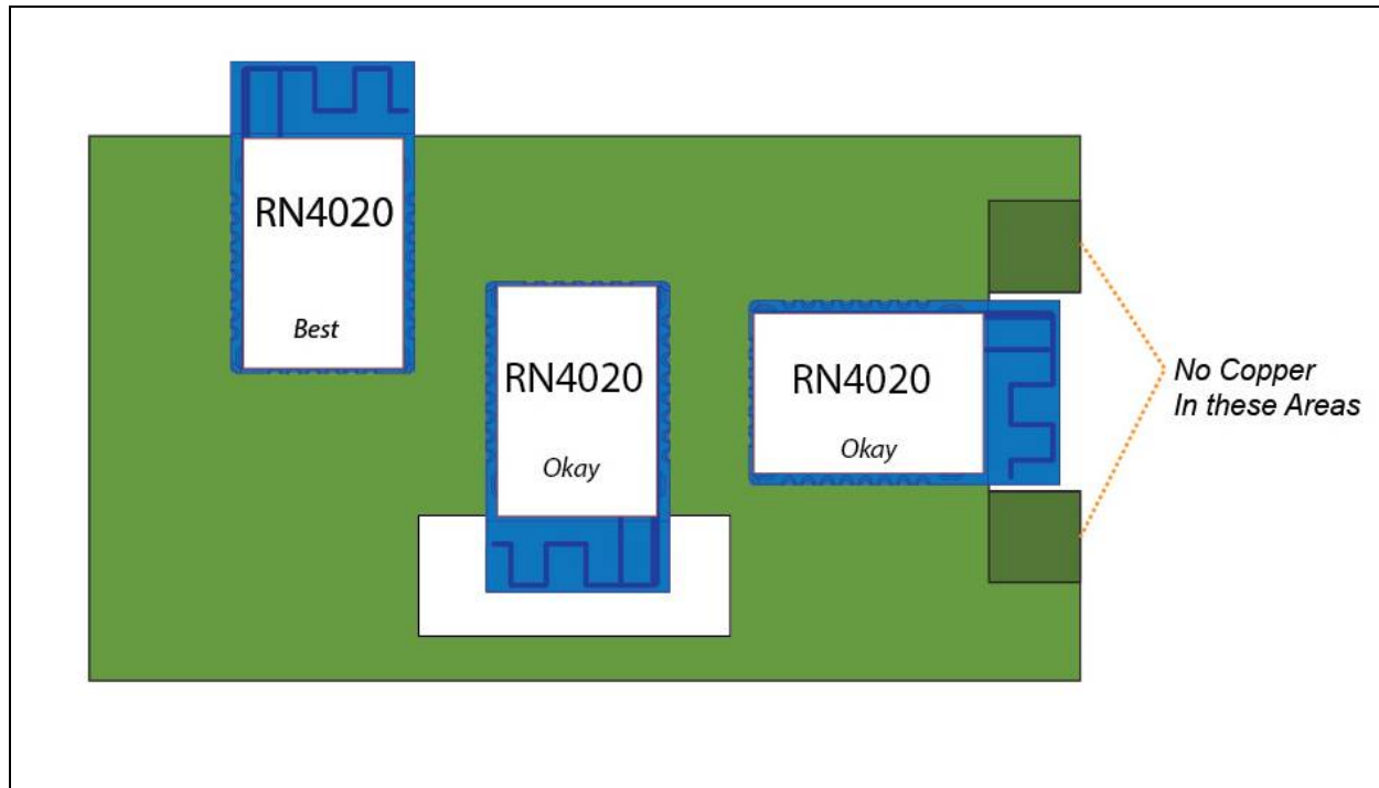
FIGURE 4-4: RN4020 HOST PCB EXAMPLE LAYOUT
