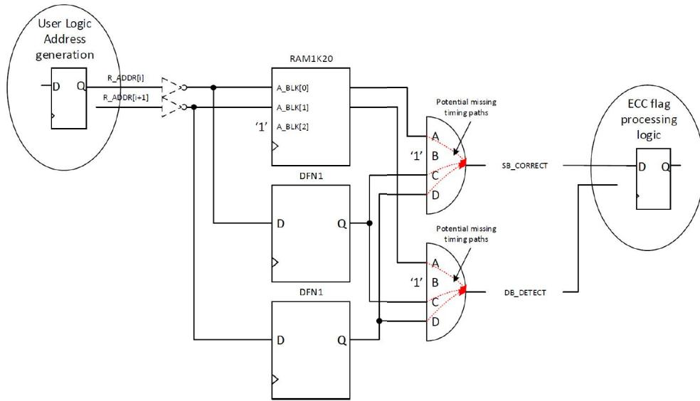
Additionally, for RTG4, combinational cells tie-offs ("1" or "0") can also occur when:
