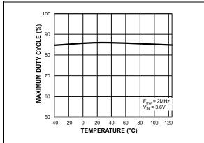
FIGURE 2-5: Maximum Duty Cycle vs. Temperature.
