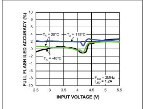
FIGURE 2-12: Full Flash ILED Accuracy vs. Input Voltage.
