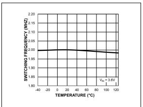
FIGURE 2-4: Switching Frequency vs. Temperature.
