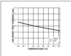
FIGURE 2-7: LED Short Test Current vs. Temperature.
