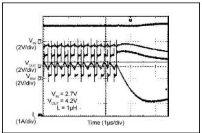
FIGURE 2-29: Switch Current Limit.
