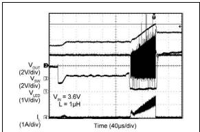
FIGURE 2-23: V<sub>OUT</sub> Overvoltage Protection (Overvoltage during Start-up).
