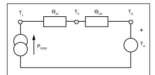
FIGURE 7-2: Series Thermal Resistance Circuit.
