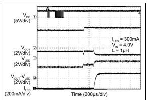
FIGURE 2-16: Torch Mode Turn-On Sequence (Linear Mode).
