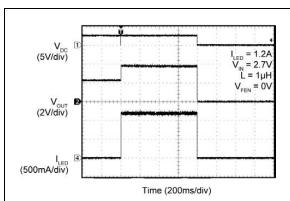
**FIGURE 2-21:** Load Disconnect at Shutdown ( $V_{IN} = 2.7V$ ).
