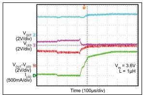
FIGURE 2-25: Load Transient (Torch 63 mA to Flash 1.2A).
