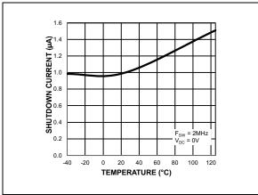
FIGURE 2-1: Shutdown Current vs. Temperature.
