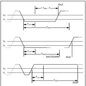
FIGURE 5-1: Abort, Shutdown and Idle Timing Waveforms.
