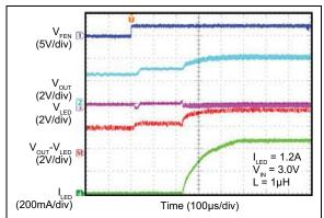
FIGURE 2-13: Flash Mode Turn-On Sequence (Boost Mode).
