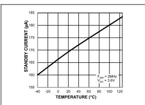
FIGURE 2-2: Standby Current vs. Temperature.
