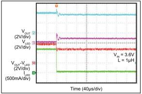
FIGURE 2-26: Load Transient (Flash 1.2A to Torch 63 mA).
