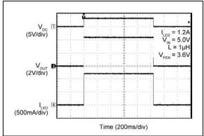
FIGURE 2-22: Load Disconnect at Shutdown ( $V_{IN} = 5.0V$ ).
