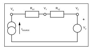
FIGURE 7-1: Series Electrical Resistance Circuit.
