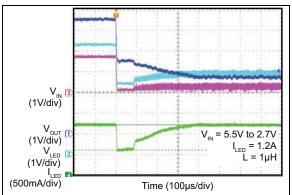
FIGURE 2-28: Line Transient (V<sub>IN</sub> Changes from 5.5V to 2.7V).
