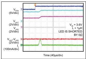
**FIGURE 2-19:** LED Short-Circuit Protection (LED is Shorted by  $\Omega\Omega$ ).
