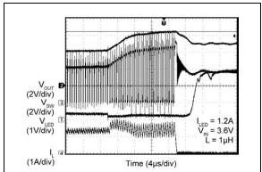
**FIGURE 2-24:** V<sub>OUT</sub> Overvoltage Protection (Overvoltage after Start-up).
