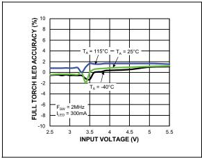
FIGURE 2-11: Full Torch ILED Accuracy vs. Input Voltage.
