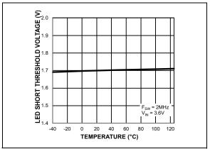
FIGURE 2-6: LED Short Threshold Voltage vs. Temperature.
