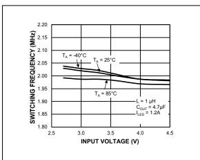
FIGURE 2-8: Boost Switching Frequency vs. Input Voltage.
