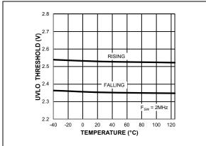
FIGURE 2-3: UVLO Threshold vs. Temperature.
