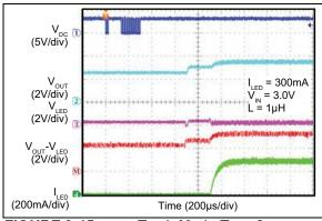
FIGURE 2-15: Torch Mode Turn-On Sequence (Boost Mode).
