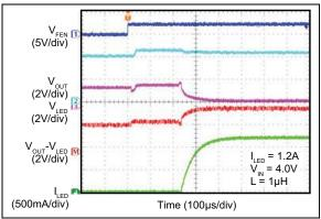
FIGURE 2-14: Flash Mode Turn-On Sequence (Linear Mode).
