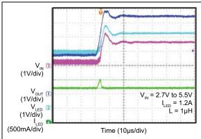
FIGURE 2-27: Line Transient (V<sub>IN</sub> Changes from 2.7V to 5.5V).
