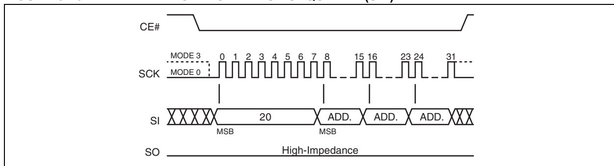
FIGURE 5-20: 4 KBYTE SECTOR-ERASE SEQUENCE (SPI)
