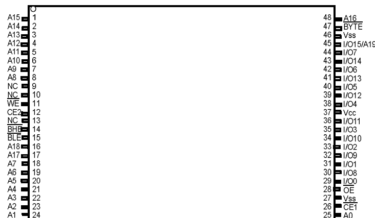
Figure 3. 48-pin TSOP I pinout (Top View) [1, 3]
