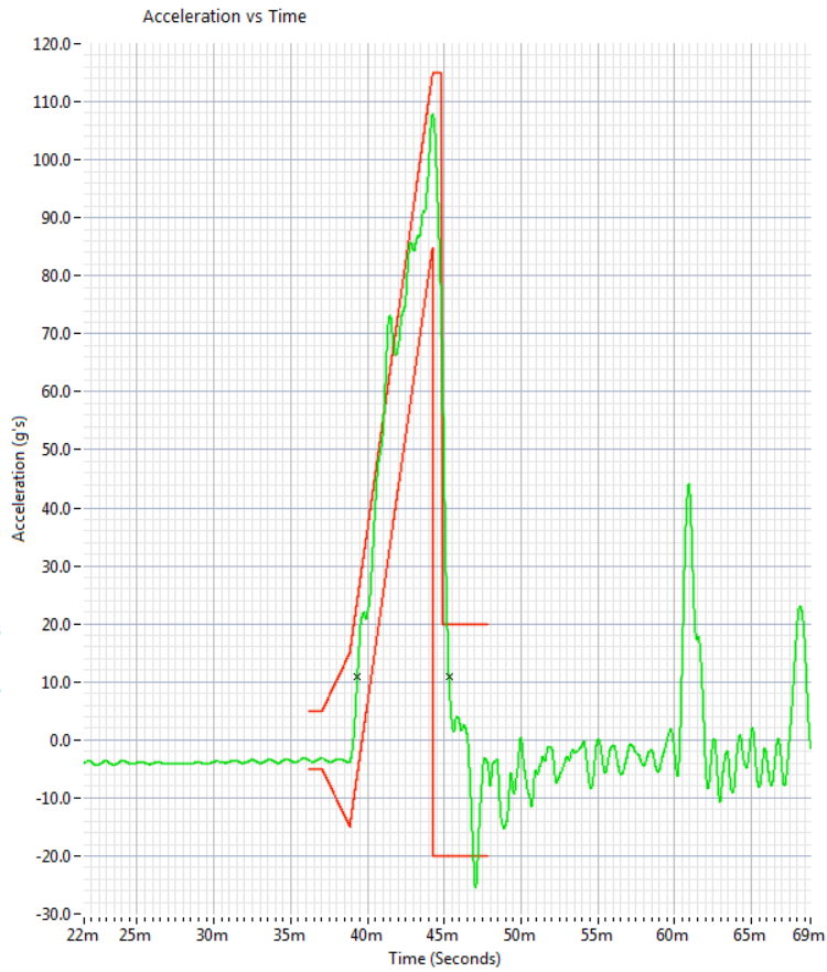
Figure 5 Mechanical Shock Half Sine Profile
