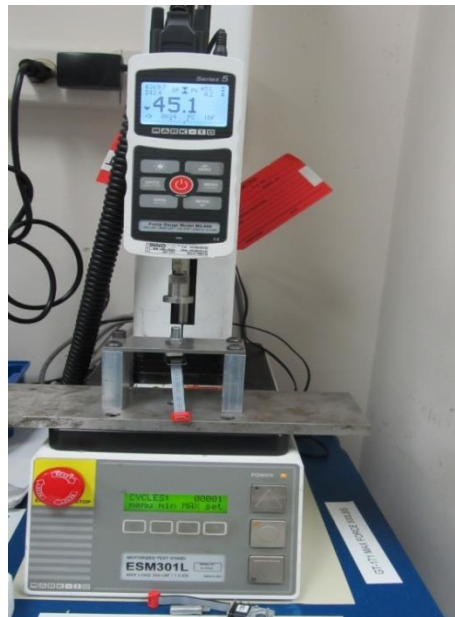
Figure 14 - Push Out Force Test Setup
