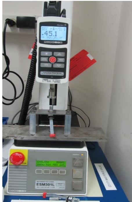
Figure 13 - Pull Out Test Setup
