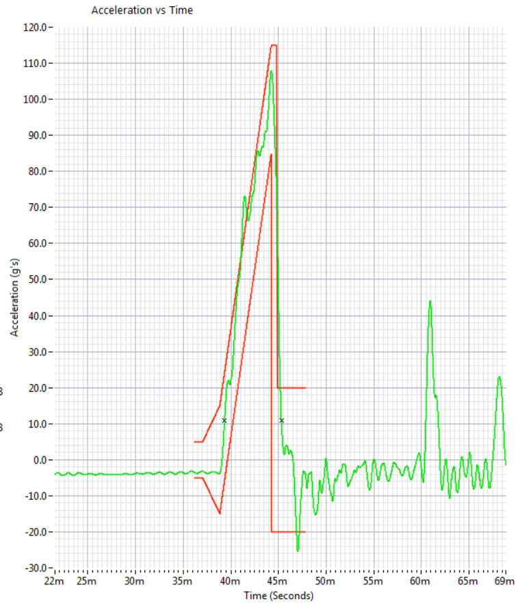
Figure 4 - Mechanical Shock Sawtooth Profile
