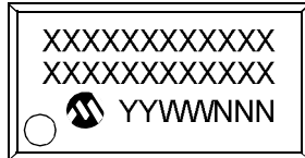
28-Lead SSOP (5.30 mm)
