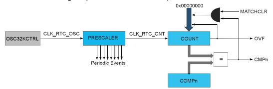
Figure 27-2. RTC Block Diagram (Mode 1 — 16-Bit Counter)
