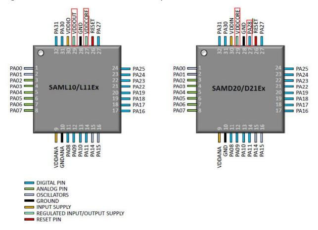
Figure 54-1. TQFP-32 and QFN-32 Pin-to-Pin Comparison
