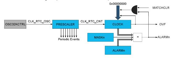
Figure 27-4. RTC Block Diagram (Tamper Detection Use Case)
