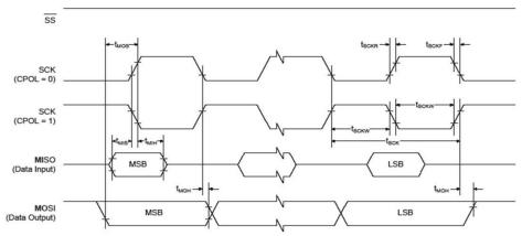
Figure 47-3. SPI Timing Requirements in Slave Mode
