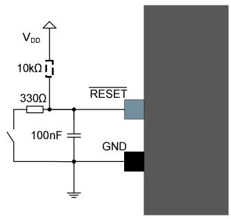
Figure 50-6. External Reset Circuit Schematic (EFT Immunity Enhancement)
