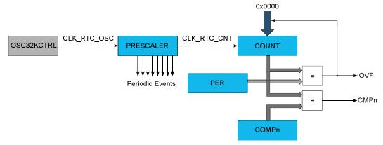
Figure 27-3. RTC Block Diagram (Mode 2 — Clock/Calendar)
