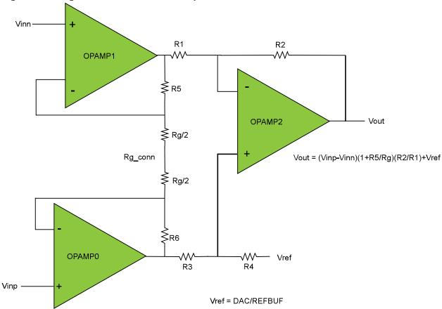
Figure 44-9. High Gain Instrumentation amplifier
