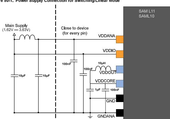
Figure 50-1. Power Supply Connection for Switching/Linear Mode
