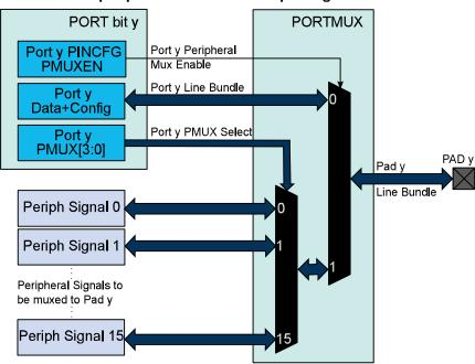
Figure 32-3. Overview of the peripheral functions multiplexing
