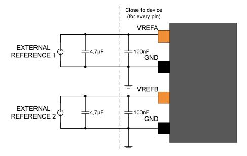
Figure 50-4. External Analog Reference Schematic With One Reference
