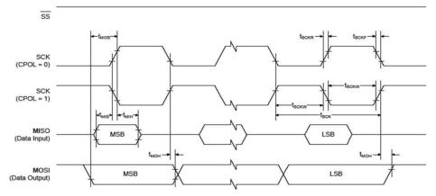
Figure 46-6. SPI Timing Requirements in Slave Mode
