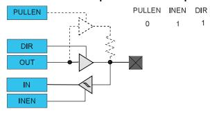
Figure 32-8. I/O Configuration - Output with Pull
