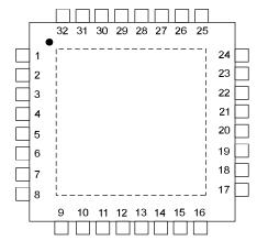
Figure 4-4. SAM L10/L11 32-pin WLCSP Pinout
