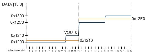
Figure 43-2. DAC Conversions in Dithering Mode (CTRLB.LEFTADJ=1)
