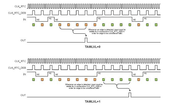
Figure 27-8. Edge Detection with Asynchronous Stability Debouncing
