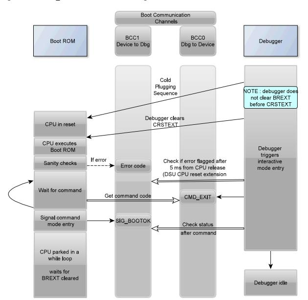
Figure 14-9. CMD\_EXIT to Park mode flow diagram
