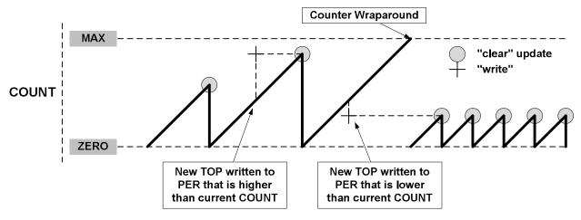
A counter wraparound can occur in any operation mode when up-counting without buffering, see Figure 38-8.
