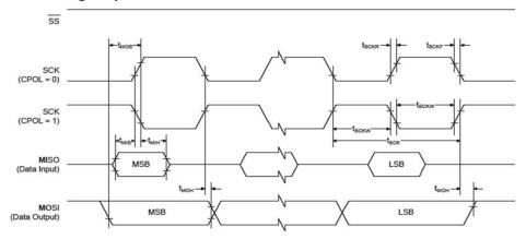
Figure 47-5. SPI Timing Requirements in Slave Mode
