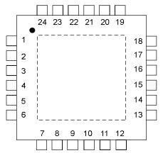
Figure 4-2. SAM L10/L11 24-pin SSOP Pinout
