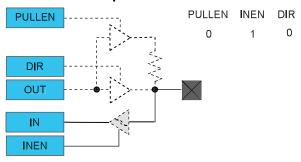
Figure 32-5. I/O Configuration - Input with Pull
