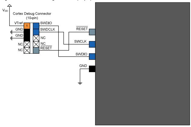
**Table 50-7. Cortex Debug Connector (10-pin)**
