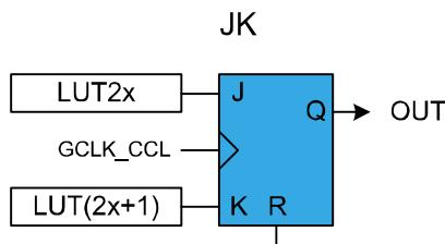
When the even LUT is disabled (LUTCTRL0.ENABLE=0 / LUTCTRL2.ENABLE=0), the flip-flop is asynchronously cleared. The reset command (R) is kept enabled for one APB clock cycle. In all other cases, the flip-flop output (OUT) is refreshed on rising edge of the GCLK\_CCL, as shown in [Table 37-3](#).
