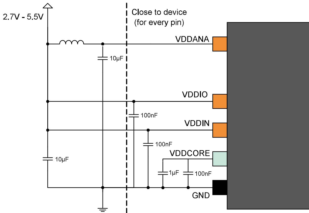
**Figure 50-2. Dual Power Supply Schematic**
