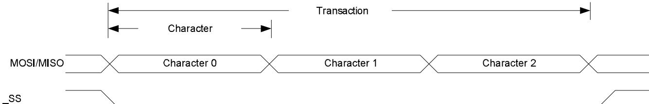
The SPI master must pull the slave select line ( $\overline{SS}$ ) of the desired slave low to initiate a transaction. The master and slave prepare data to send via their respective shift registers, and the master generates the serial clock on the SCK line.
