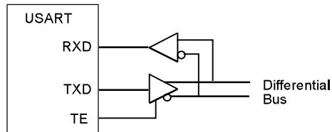
The TE pin will remain high for the complete frame including stop bit(s). If a Guard Time is programmed in the Control C register (CTRLC.GTIME), the line will remain driven after the last character completion. The following figure shows a transfer with one stop bit and  $\text{CTRLC.GTIME}=3$ .
