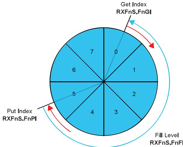
When reading from an Rx FIFO, Rx FIFO Get Index RXFnS.FnGI • FIFO Element Size has to be added to the corresponding Rx FIFO start address RXFnC.FnSA.
