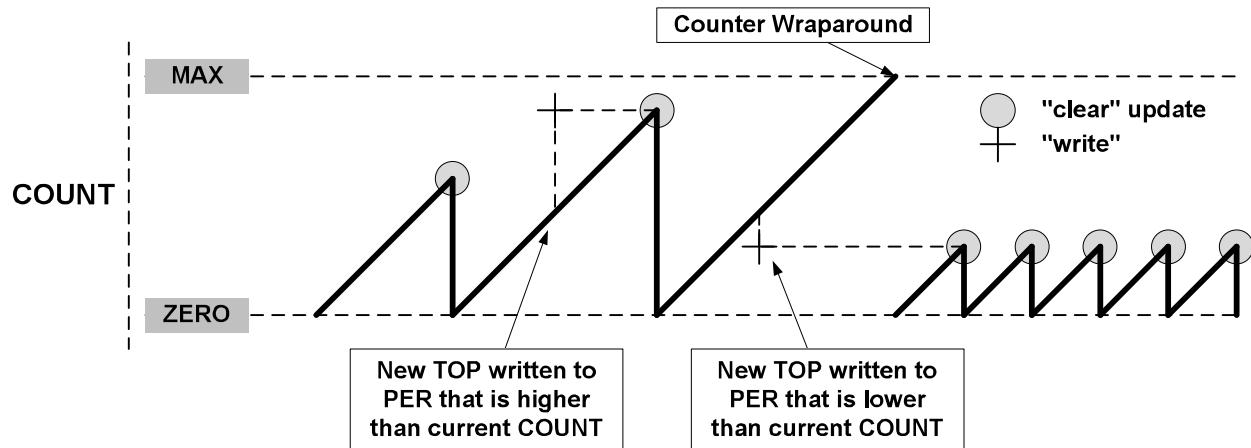
A counter wraparound can occur in any operation mode when up-counting without buffering, see [Figure 35-8](#).
