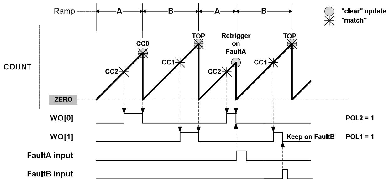
**Figure 36-21. RAMP2 Critical Operation With 2 Channels**
