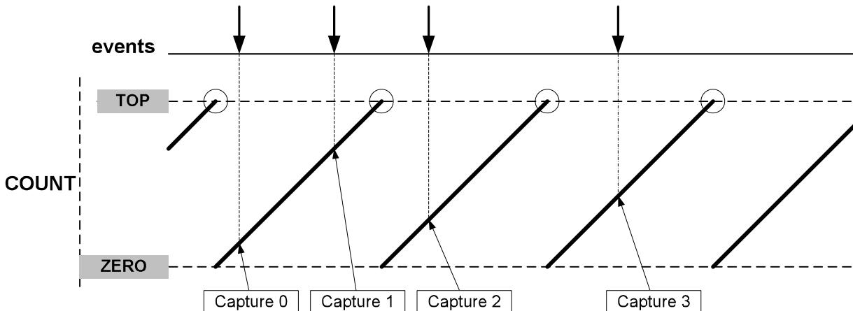
The TC can detect capture overflow of the input capture channels: When a new capture event is detected while the Capture Interrupt flag (INTFLAG.MC<sub>x</sub>) is still set, the new timestamp will not be stored and INTFLAG.ERR will be set.
