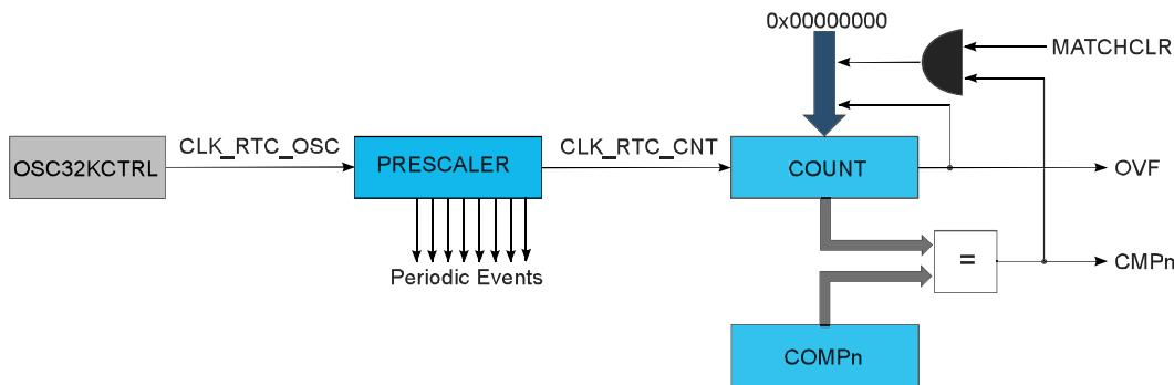
**Figure 24-2. RTC Block Diagram (Mode 1 — 16-Bit Counter)**
