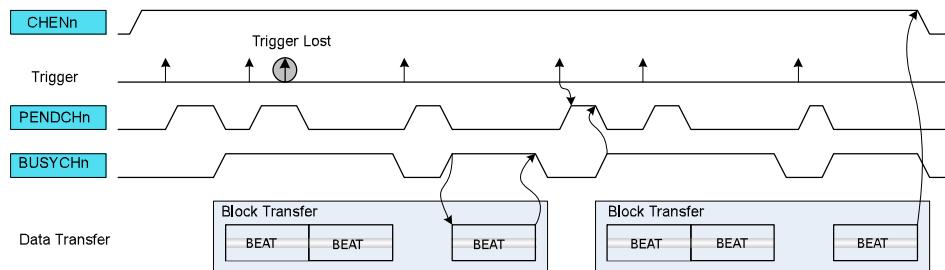
**Block Trigger Action**
