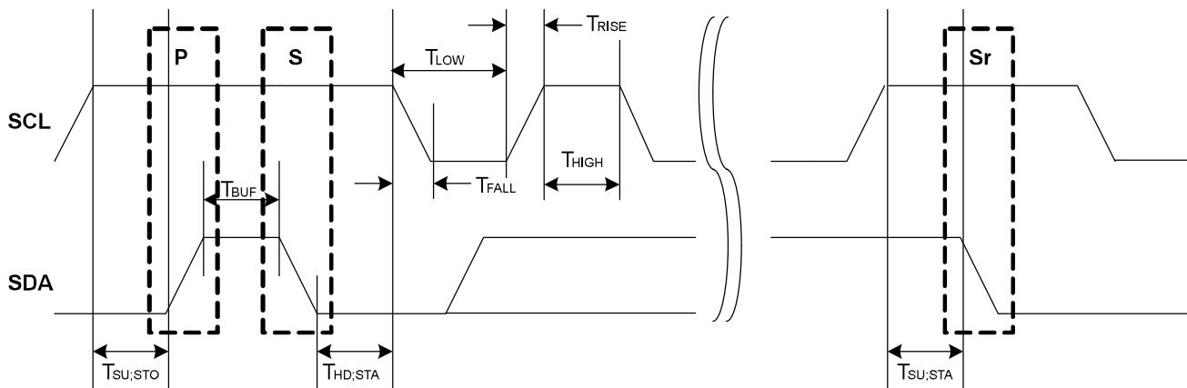
The following parameters are timed using the SCL low time period  $T_{LOW}$ . This comes from the Master Baud Rate Low bit group in the Baud Rate register (BAUD.BAUDLOW). When BAUD.BAUDLOW=0, or the Master Baud Rate bit group in the Baud Rate register (BAUD.BAUD) determines it.
