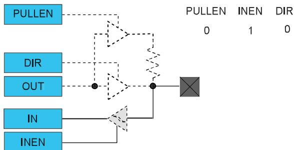
**Figure 28-5. I/O Configuration - Input with Pull**
