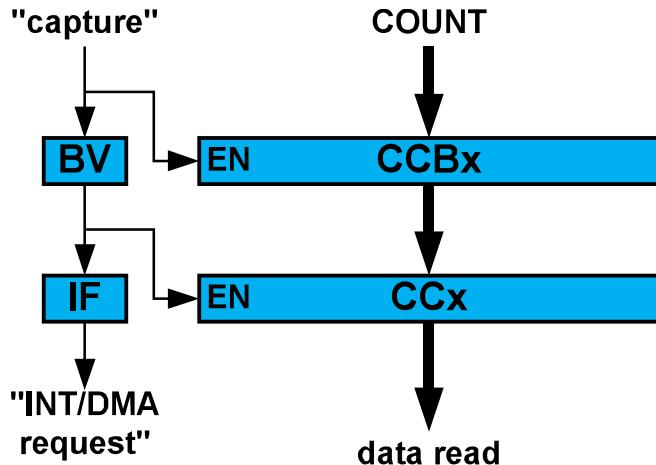
For input capture, the buffer register and the corresponding CC<sub>x</sub> act like a FIFO. When CC<sub>x</sub> is empty or read, any content in CCBUF<sub>x</sub> is transferred to CC<sub>x</sub>. The buffer valid flag is passed to set the CC<sub>x</sub> interrupt flag (IF) and generate the optional interrupt, event or DMA request. The CCBUF<sub>x</sub> register value can't be read, all captured data must be read from CC<sub>x</sub> register.
