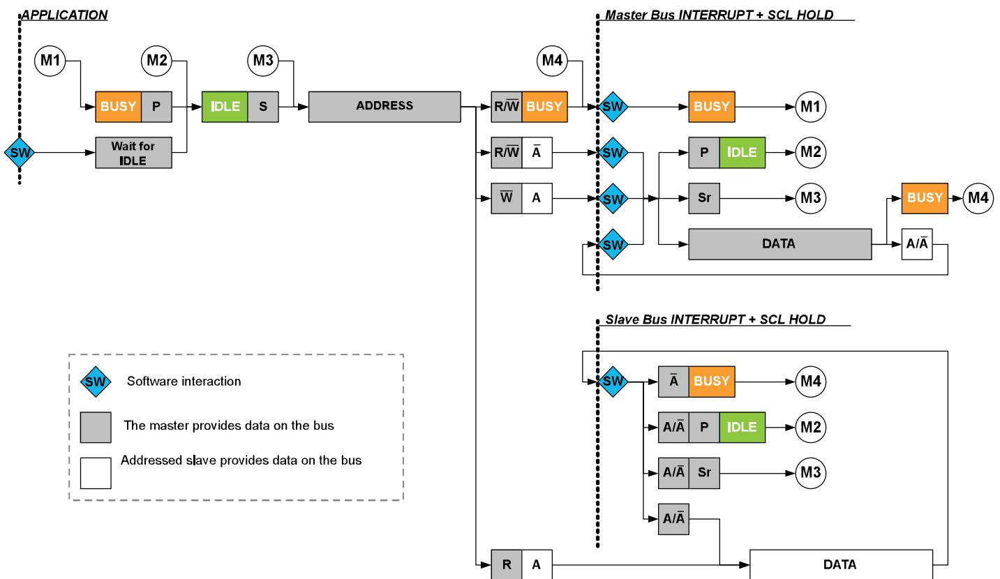
In the second strategy (CTRLA.SCLSM=1), interrupts only occur after the ACK bit, as in [Master Behavioral Diagram \(SCLSM=1\)](#). This strategy can be used when it is not necessary to check DATA before acknowledging.
