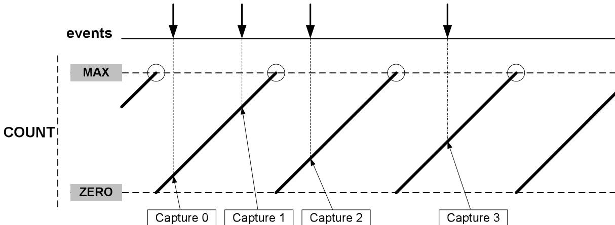
For input capture, the buffer register and the corresponding CCx act like a FIFO. When CCx is empty or read, any content in CCBUFx is transferred to CCx. The buffer valid flag is passed to set the CCx interrupt flag (IF) and generate the optional interrupt, event or DMA request. CCBUFx register value can't be read, all captured data must be read from CCx register.
