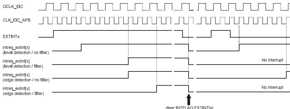
The detection latency depends on the detection mode.
