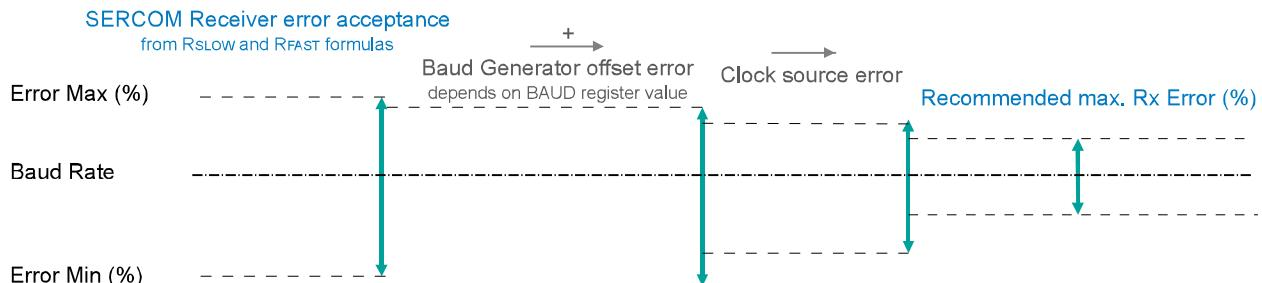
The recommendation values in the table above accommodate errors of the clock source and the baud generator. The following figure gives an example for a baud rate of 3Mbps:
