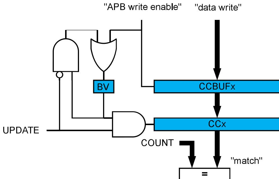
Both the registers (PATT/WAVE/PER/CCx) and corresponding buffer registers (PATTBUF/WAVEBUFV/PERBUF/CCBUF<sub>x</sub>) are available in the I/O register map, and the double buffering feature is not mandatory. The double buffering is disabled by writing a '1' to CTRLSET.LUPD.
