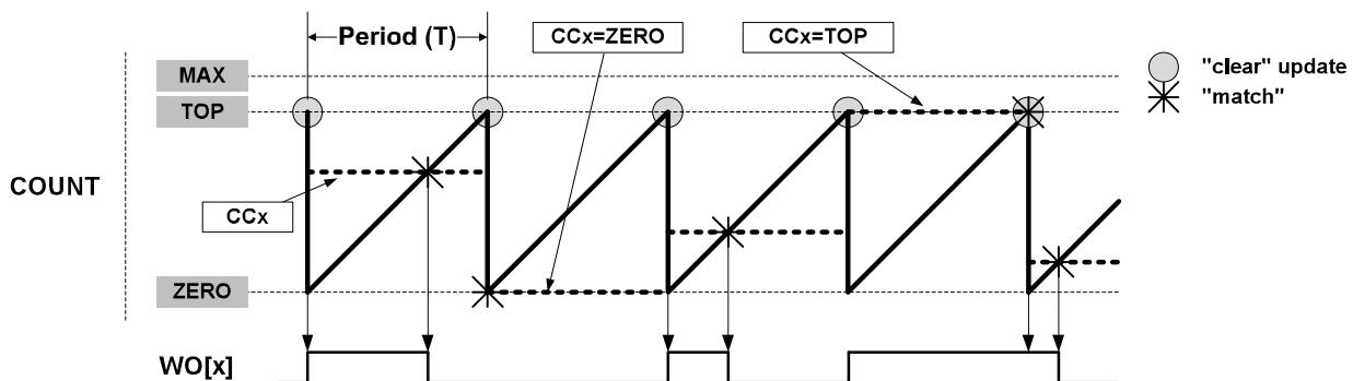
The following equation calculates the exact resolution for a single-slope PWM ( $R_{\text{PWM\_SS}}$ ) waveform:
