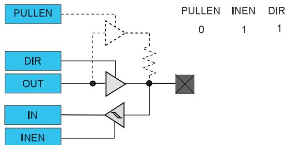
**Figure 28-8. I/O Configuration - Output with Pull**
