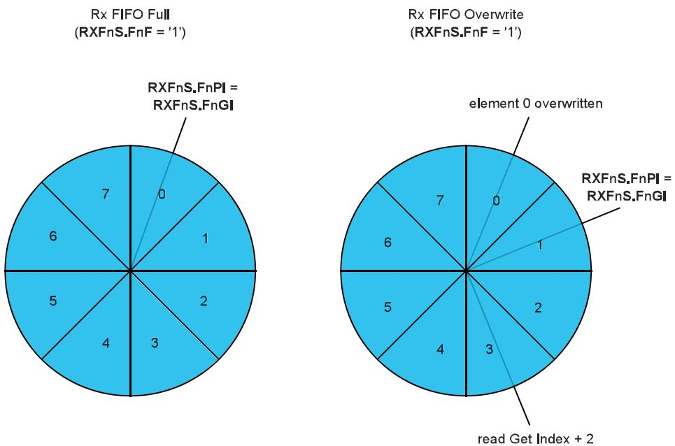
After reading from the Rx FIFO, the number of the last element read has to be written to the Rx FIFO Acknowledge Index  $\text{RXFnA.FnA}$ . This increments the get index to that element number. In case the put index has not been incremented to this Rx FIFO element, the Rx FIFO full condition is reset ( $\text{RXFnS.FnF} = '0'$ ).
