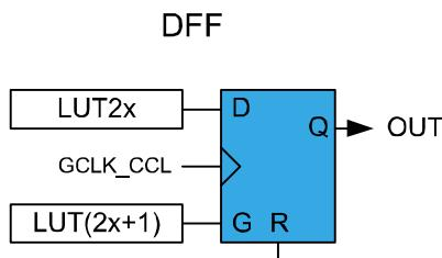
When the even LUT is disabled (LUTCTRL0.ENABLE=0 / LUTCTRL2.ENABLE=0), the flip-flop is asynchronously cleared. The reset command (R) is kept enabled for one APB clock cycle. In all other cases, the flip-flop output (OUT) is refreshed on rising edge of the GCLK\_CCL, as shown in [Table 37-2](#).
