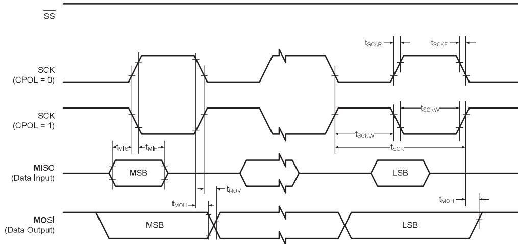
**Figure 45-8. SPI Timing Requirements in Slave Mode**
