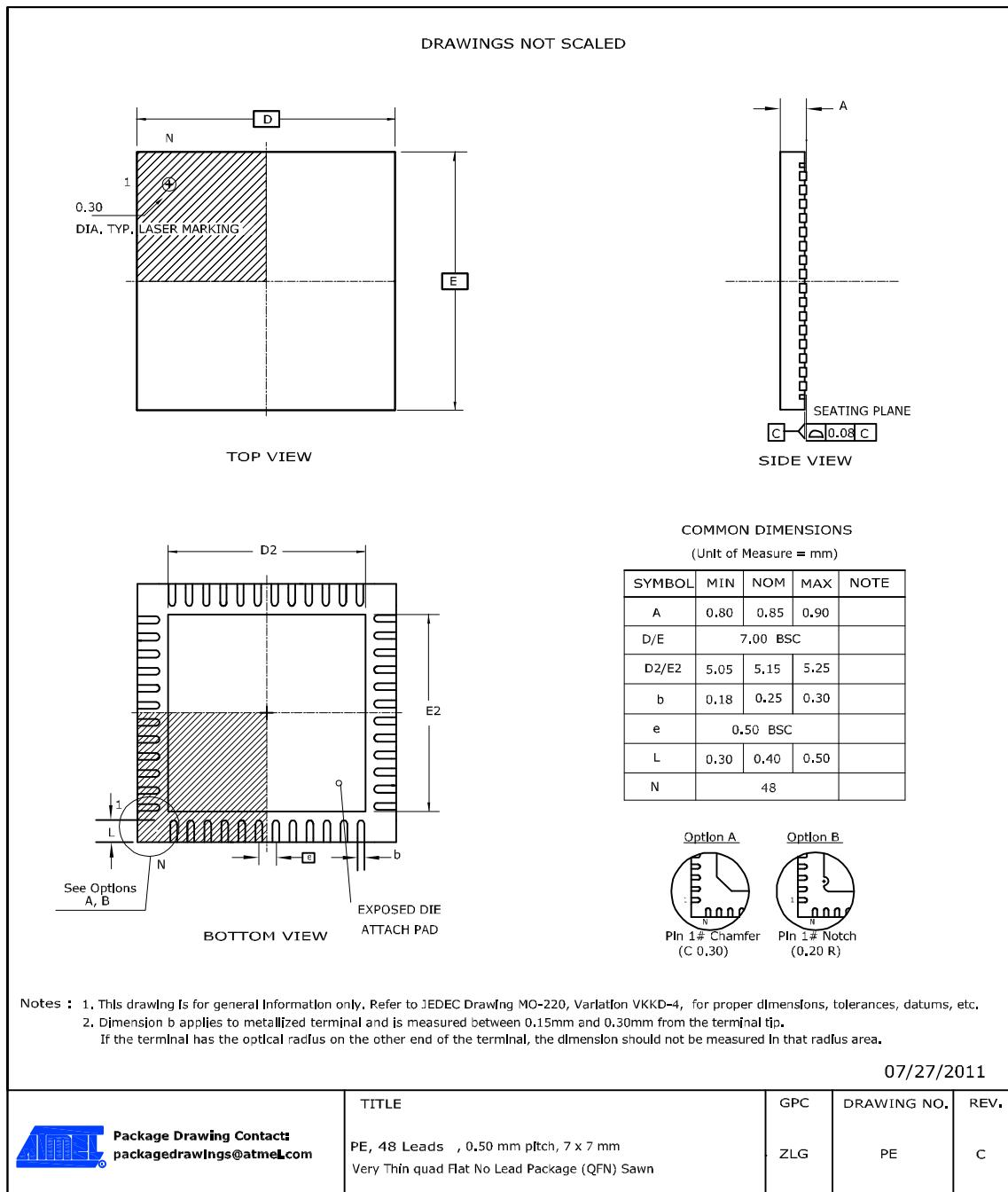
**Note:** The exposed die attach pad is not connected electrically inside the device.
