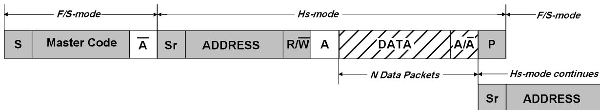
Transmitting in High-speed mode requires the I<sup>2</sup>C master to be configured in High-speed mode (CTRLA.SPEED=0x2) and the SCL clock stretch mode (CTRLA.SCLSM) bit set to '1'.
