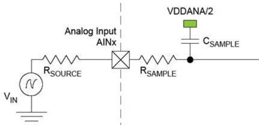
The minimum sampling time  $t_{\text{samplehold}}$  for a given  $R_{\text{source}}$  can be found using this formula:
