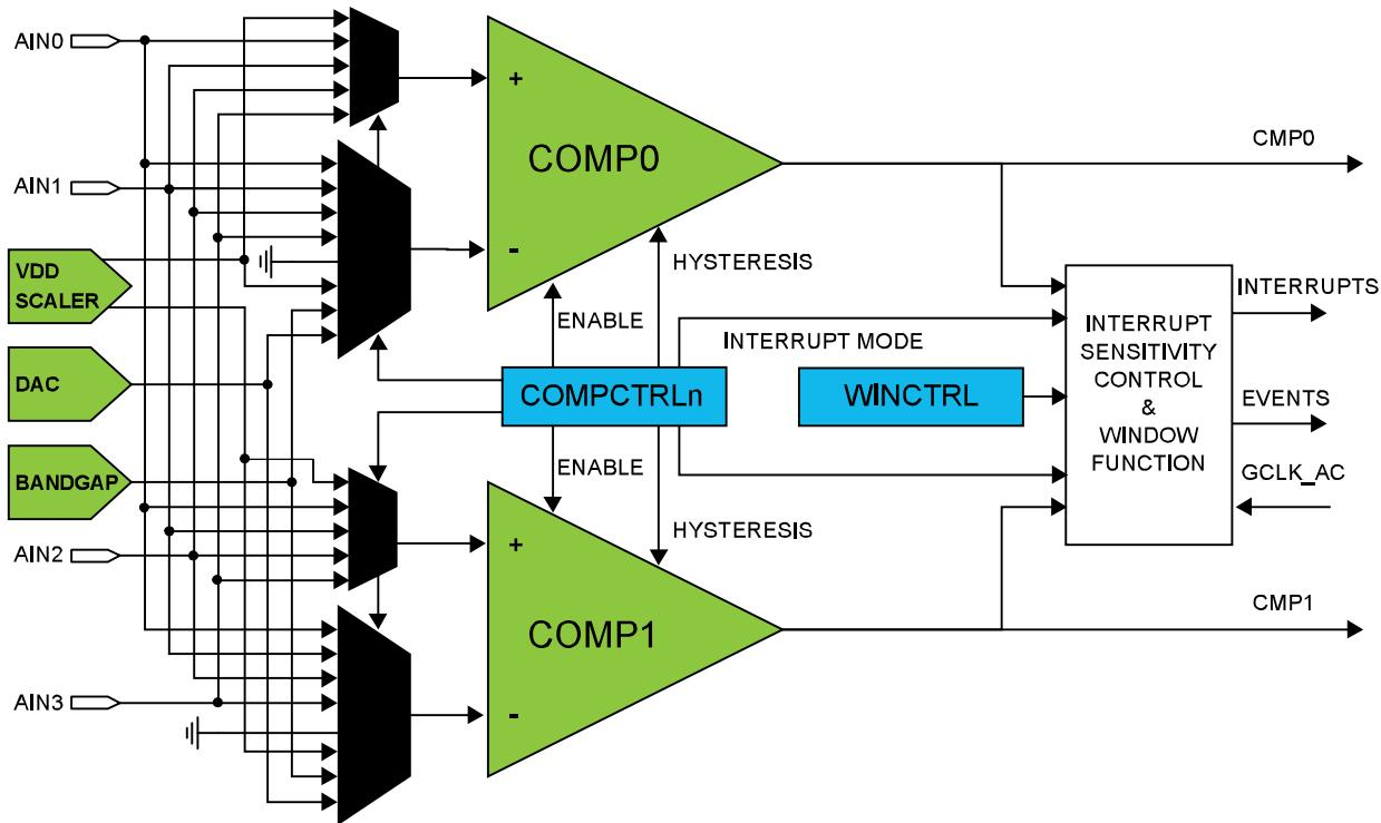
Figure 40-2. Analog Comparator Block Diagram (Second Pair)
