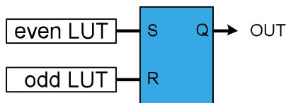
When the even LUT is disabled LUTCTRL0.ENABLE=0 / LUTCTRL2.ENABLE=0), the latch output will be cleared. The R-input is forced enabled for one more APB clock cycle and S-input to zero. In all other cases, the latch output (OUT) is refreshed as shown in [Table 37-5](#).
