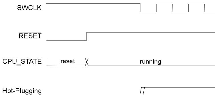
The presence of a debugger probe is detected when either Hot-Plugging or Cold-Plugging is detected. Once detected, the Debugger Present bit of the Status B register (STATUSUSB.DBGPRES) is set. For security reasons, Hot-Plugging is not available when the device is protected by the NVMCTRL security bit.
