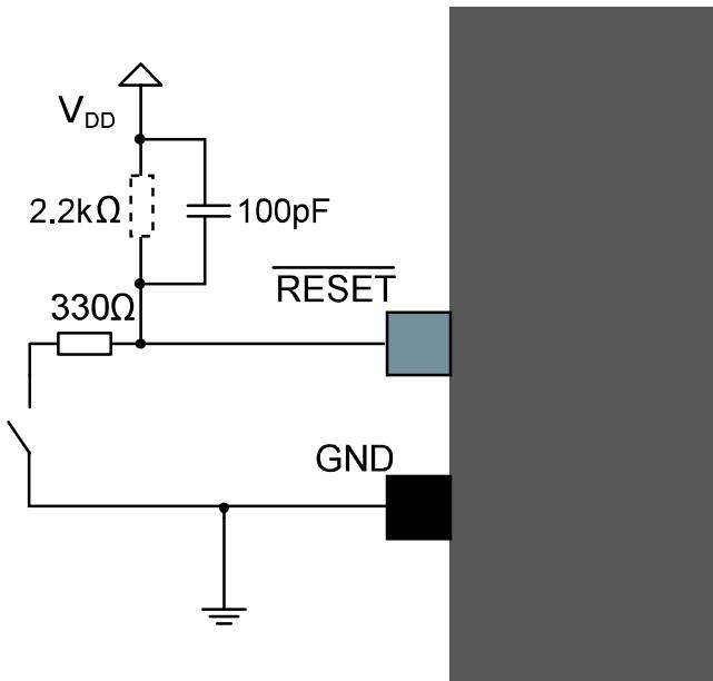
A pull-up resistor makes sure that the reset does not go low and unintentionally causing a device reset. An additional resistor has been added in series with the switch to safely discharge the filtering capacitor, i.e. preventing a current surge when shorting the filtering capacitor which again can cause a noise spike that can have a negative effect on the system.
