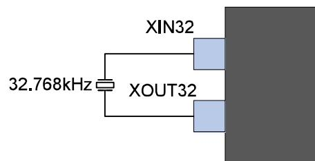
To improve accuracy and Safety Factor, the crystal datasheet can recommend adding external capacitors as shown in [Figure 50-9](#).
