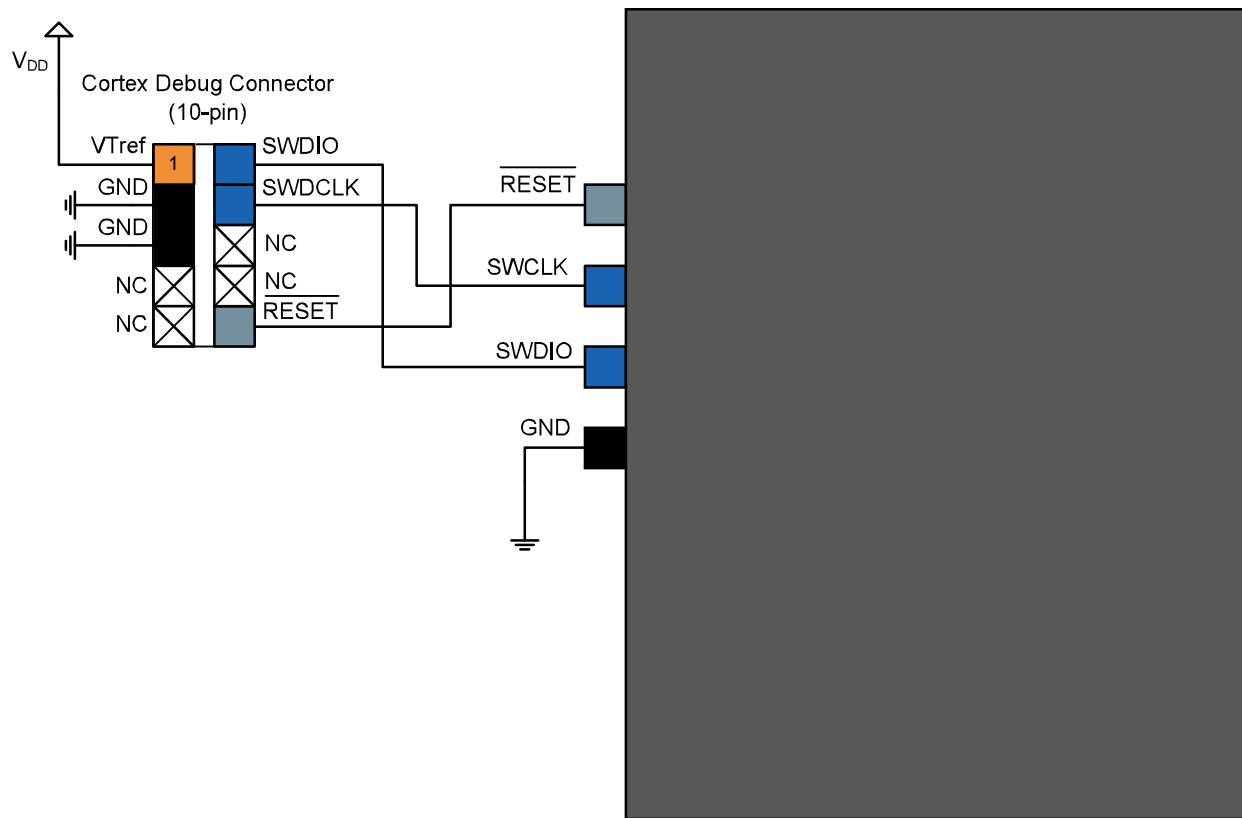
**Table 50-8. Cortex Debug Connector (10-pin)**
