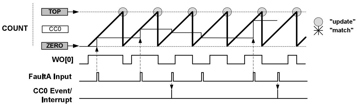
**Hardware** This is configured by writing 0x1 to the Fault n Halt mode bits in the Recoverable Fault n **Halt Action** Configuration register (FCTRLn.HALT). When enabled, the timer/counter is halted and the cycle is extended as long as the corresponding fault is present.
