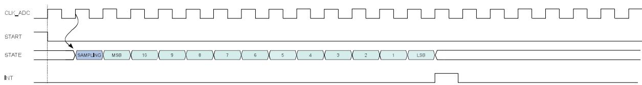
The sampling time can be increased by using the Sampling Time Length bit group in the Sampling Time Control register (SAMPCTRL.SAMPLEN). As example, the next figure is showing the timing conversion with sampling time increased to six CLK\_ADC cycles.
