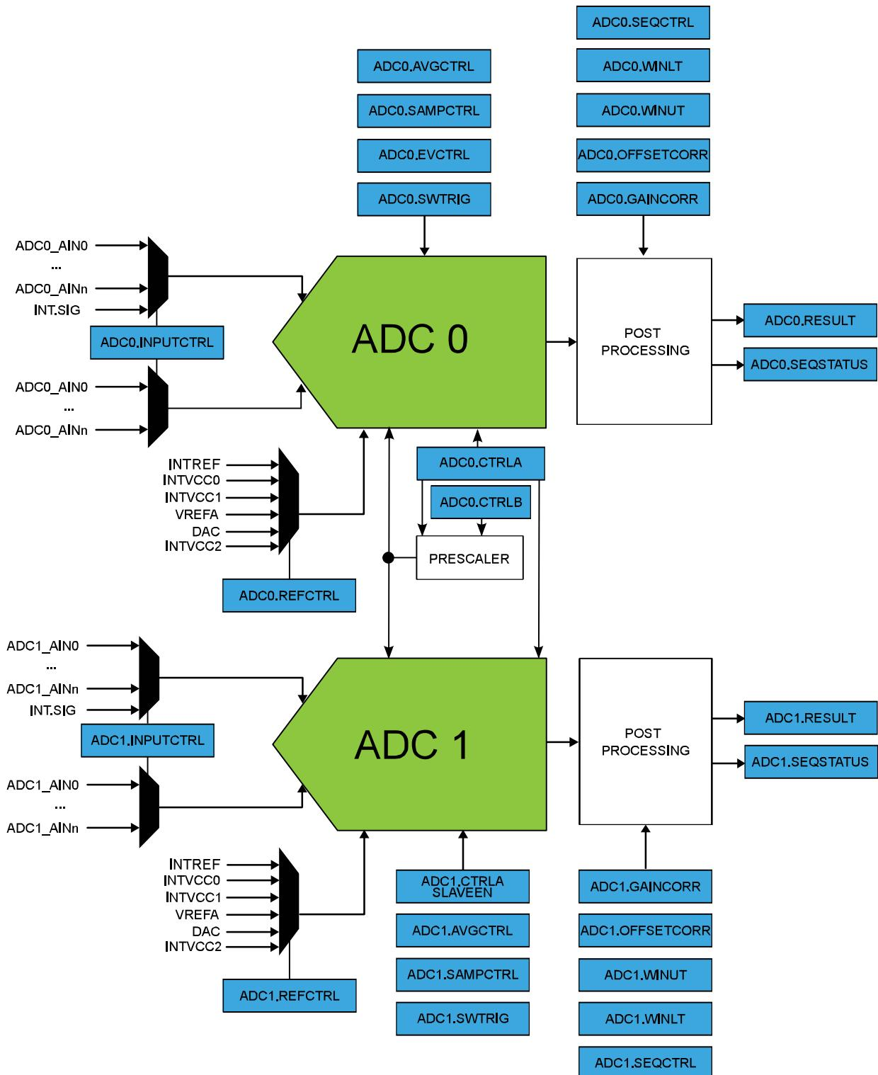
In this mode of operation, the slave ADC is enabled by accessing the CTRLA register of master ADC. In the same way, the master ADC event inputs will be automatically routed to the slave ADC, meaning that the input events configuration must be done in the master ADC (ADC0.EVCTRL).
