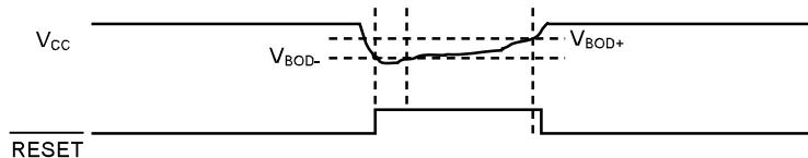
Enabling the BODVDD hysteresis by writing the Hysteresis bit in the BODVDD register (BODVDD.HYST) to '1' will add hysteresis to the BODVDD threshold level.
