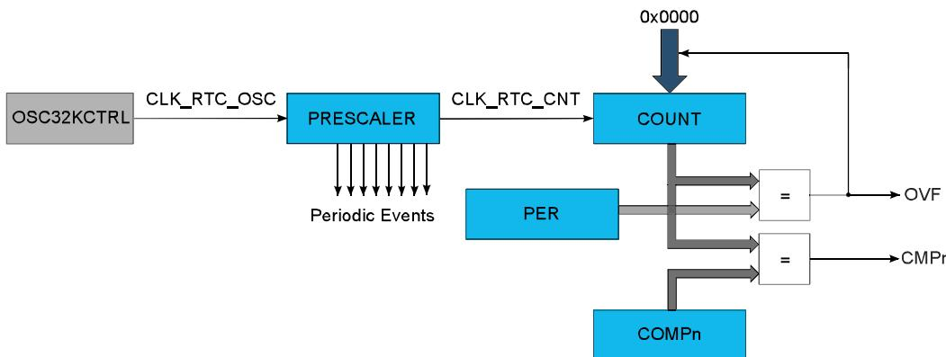
**Figure 24-3. RTC Block Diagram (Mode 2 — Clock/Calendar)**
