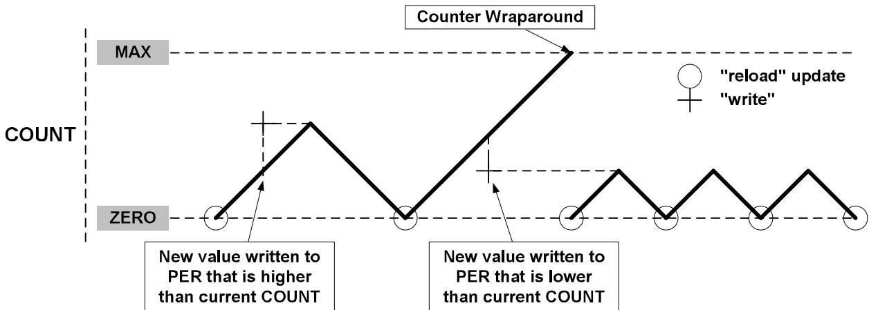
When double buffering is used, the buffer can be written at any time and the counter will still maintain correct operation. The period register is always updated on the update condition, as shown in [Figure 36-13](#). This prevents wraparound and the generation of odd waveforms.
