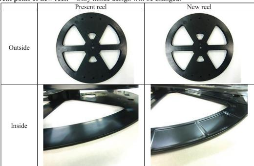
Although the new reels have different inside design as shown in the above pictures, the reel dimensions (JEITA ET-7200C), the material and the strength are the same with those of the present reels.
