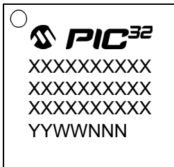
64-Lead QFN (9x9x0.9 mm) with 4.7x4.7 Exposed Pad
